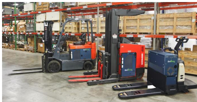
Figure 4: Fuel Cell Powered Forklifts by Plug Power Inc. Source: Plug Power Inc.
